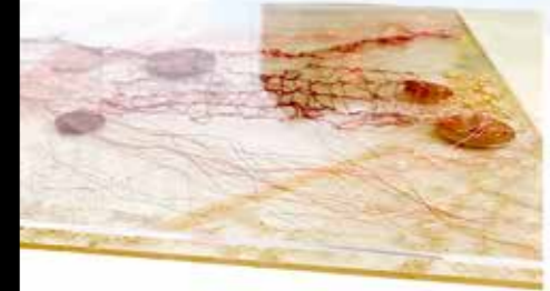
Tiles are first printed with a mono print block onto reclaimed waste Greencast acrylic offcuts cut to size by a local acrylic sheet company that donated waste offcuts for repurposing
